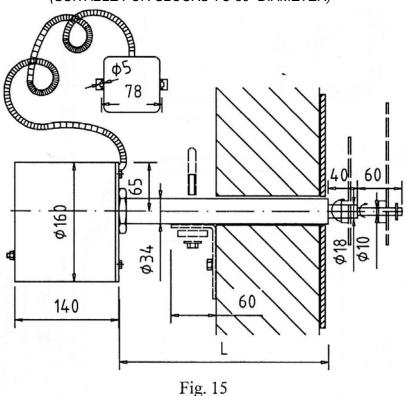
Dimension "L" is available in a number of lengths to fit most applications – contact Elderhorst Bells for information. All dimensions shown are in mm.
