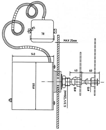
All measurements above in millimeters
