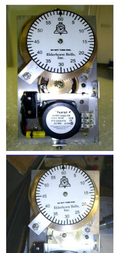
The "cam" is located between the minute dial and the "hurst" motor in the center of this photo (note: the cam profile was modified in 2007-see attached drawings). The roller on the arm of the switch follows the "cam" and switches off the motor .
