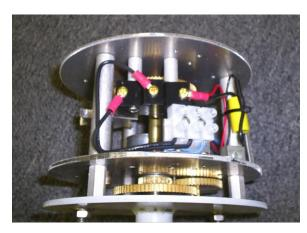
This photo – looking at the EB-106 clock movement from front to back – shows the roller switch (black, with three wires attached). This switch is mounted to the back plate of the EB-106 Clock movement with 2 bolts running through two aluminum spacers and nuts on the back side of the clock plate. Your movement may have a different switch mounting
