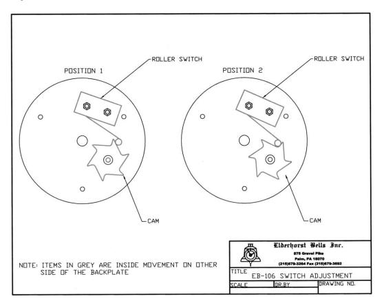
Above drawing shows the switch positioning with the "sawtooth" type cam.
