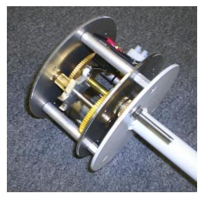
This photo shows the roller of the switch riding on the "cam". The cam in this photo is aluminum – your application may have a brass , aluminum or plastic cam with a different cam configuration
