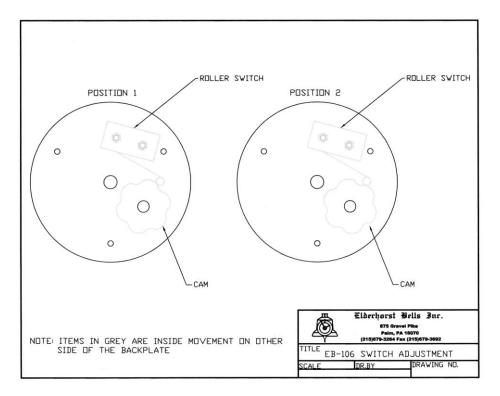
At <u>minute one</u>: an impulse will be sent out from the clock controller to the movement. The clock should advance until the roller on the switch moves to the position shown in the drawing above.
